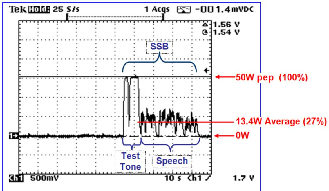
*The effects of transmission mode upon RF exposure levels on HF*
