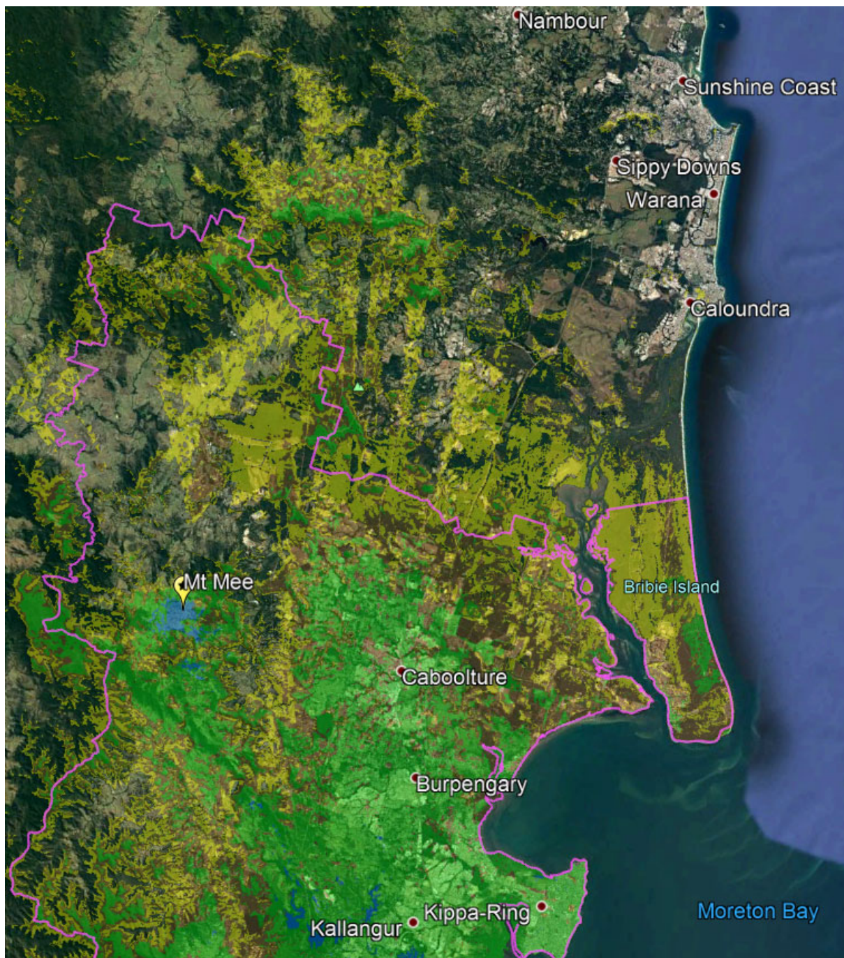
Figure 8 – Combined Mt Coot-Tha 50kW proposed Antenna (wide area) (-2deg DT) DAB+ with -10dB notch at 18 degrees centre and Mt Mee 500W proposed Antenna with -15dB back-screen reduction
