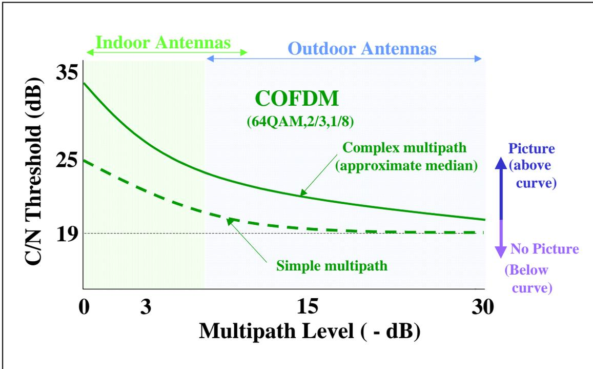
Note: The graph has been generated from multiple sources of laboratory and field trials. The indoor portion of the complex multipath curve is an extrapolation and requires verification.
