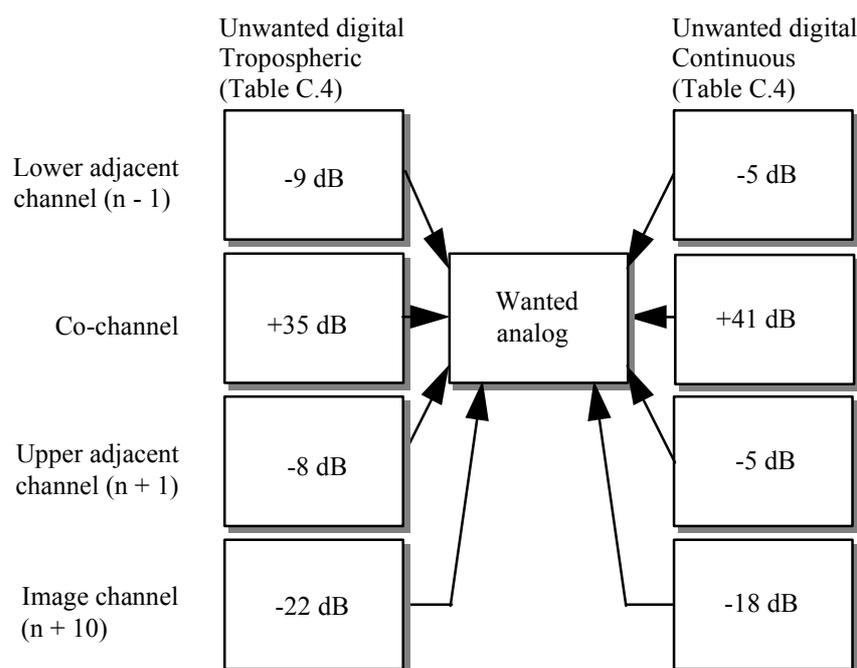
Figure C.1: Analog protection ratios for continuous and tropospheric interference
